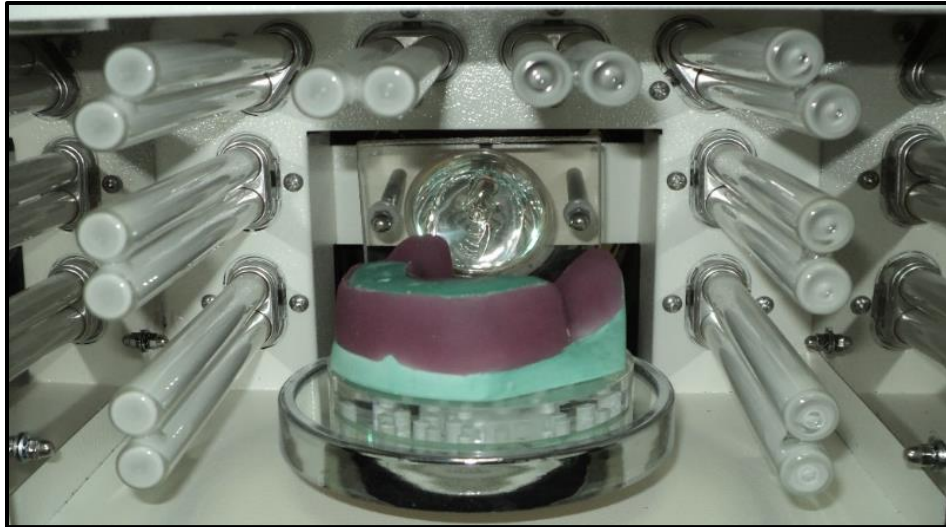
Fig.12. Curing of the acrylic resin sheet in light cure unit for a period of 5 minutes.
