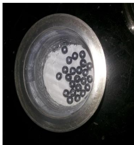
Fig 8 : Synthesized porous nanosilica along with the tungsten carbide balls
