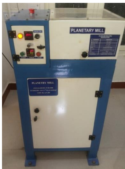
Fig 7 : Ball milling in a planetary ball mill to obtain the porous nanosilica
