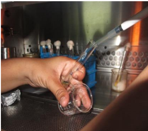
Fig 23: Sonicated bacterial suspension transferred to test tubes containing the culture media
