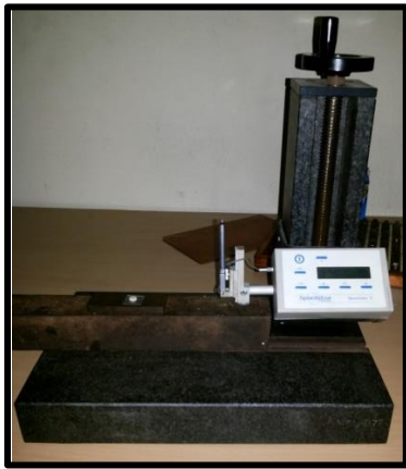
Fig 4: Standardization of specimens using Surface PROFILOMETER
