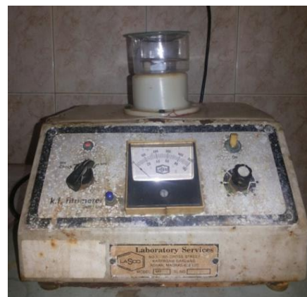
Fig 6 : Magnetic stirrer for homogenizing the mixture
