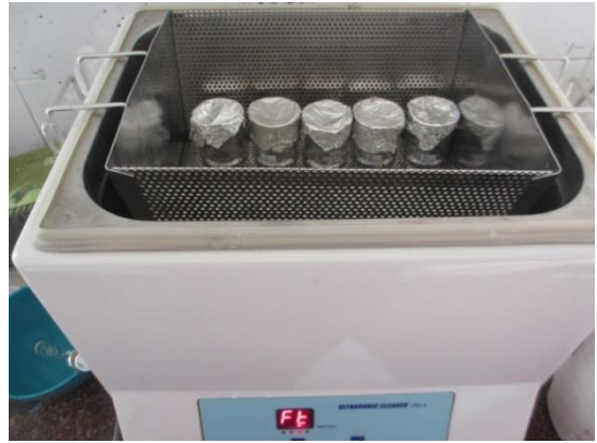
Fig 22: Adhered bacteria removed from the discs using sonication in an ultrasonic cleaner
