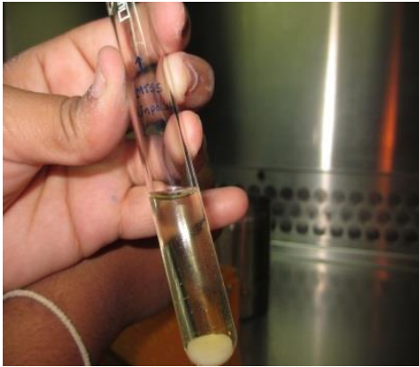
Fig 21: Specimens placed in test tubes with bacteria for biofilm formation
