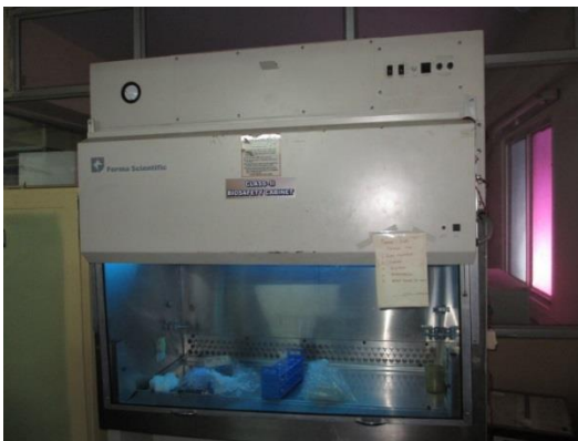
Fig 19: UV light sterilization chamber with laminar flow
