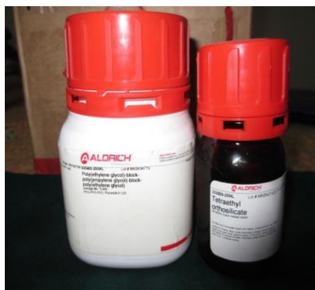
Fig 5 : TriBlock polymer- templating agent & TetraEthyl OrthoSilicate- silica source
