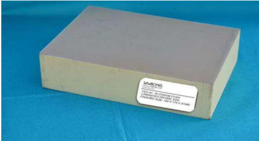
Fig 6. Sectioned Bone block with 1mm and 2mm fiber filled epoxy sheets cut into rectangular blocks of dimensions 170 X 40 X 15 mm.
