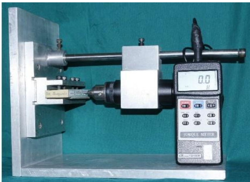
Fig 9. Aluminium apparatus with torque meter driver guide containing torque driver with MSI. Slider clamp containing bone block for insertion of MSI to quantify insertion torque.
