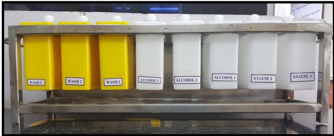
Deparaffinization stainless steel staining trough and rack
