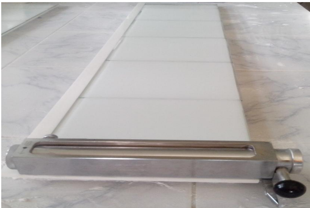
Figure-13 TLC glass plates were coated with the silica gel using spreader
