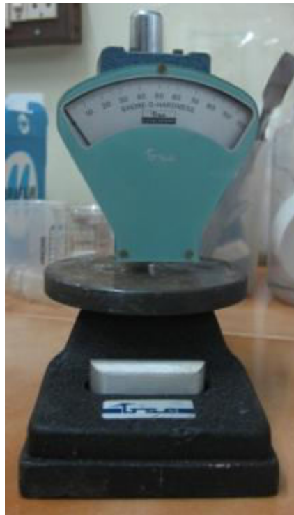
Fig.4. Shore D Durometer used to test hardness
