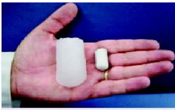
Fig: 2 i) On the left, superporous hydrogel in its dry (a) and water-swollen (b) state. ii) On the right, schematic illustration of the transit of superporous hydrogel.
