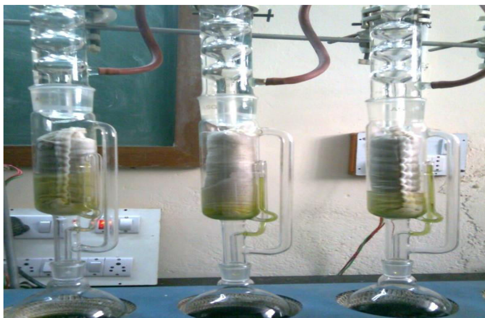
Image No. 01: Extraction using soxhlet apparatus assembly
