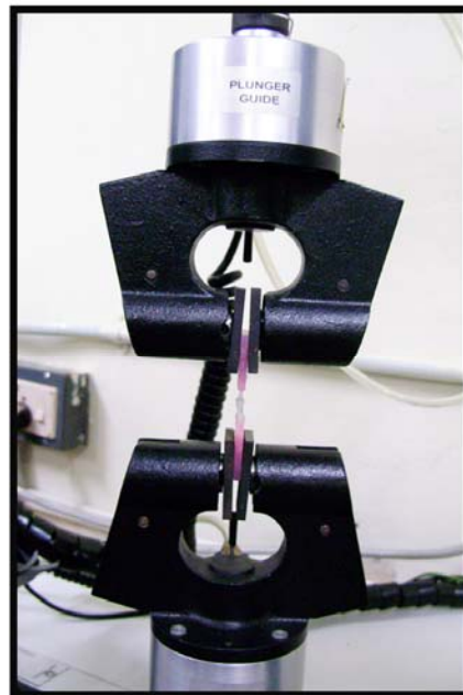
Fig - 10 Tensile bond strength testing
