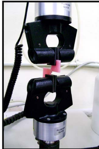
Fig -11 Shear bond strength testing
