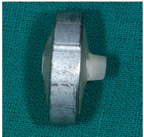
Fig.28: Porcelain veneered base metal alloy Sample embedded in the mold
