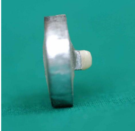
Fig.28: Porcelain veneered base metal alloy Sample embedded in the mold
