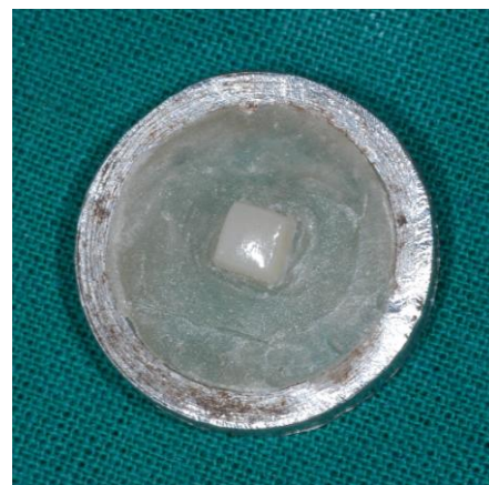
Fig.28: Porcelain veneered base metal alloy Sample embedded in the mold
