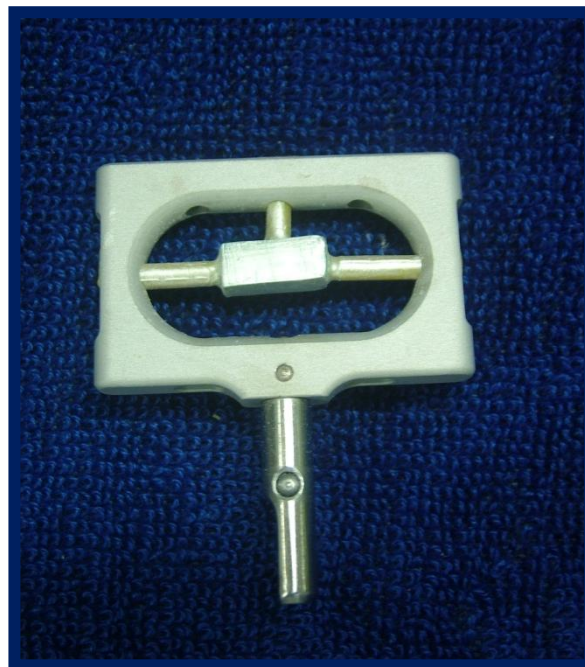
Fig. 17: Rectangular Block of CAD//CAM Wax attached to the rectangular scanning frame
