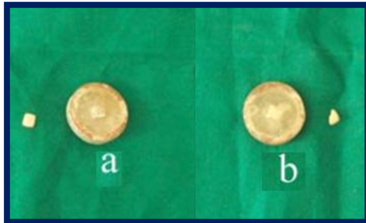
Fig.32 : Samples with fractured piece a. Porcelain veneered base metal alloy sample with fractured piece b. Porcelain veneered Zirconia sample with fractured piece
