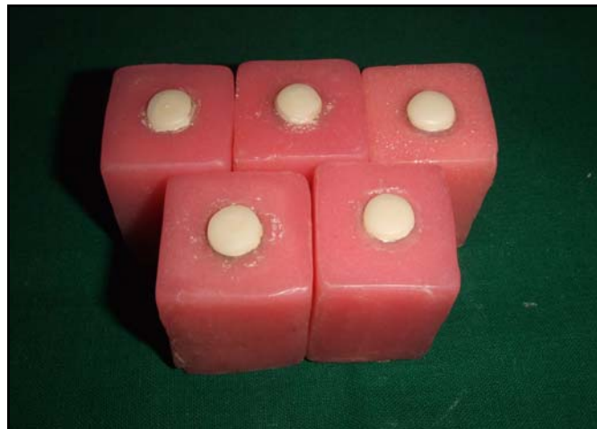
Porcelain Veneered Disc embedded in Acrylic Block
