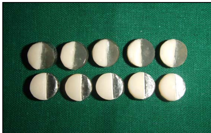
Porcelain Veneered Disc embedded in Acrylic Block
