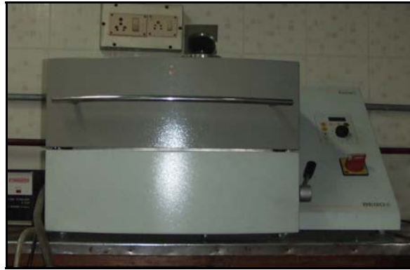
Induction casting machine
