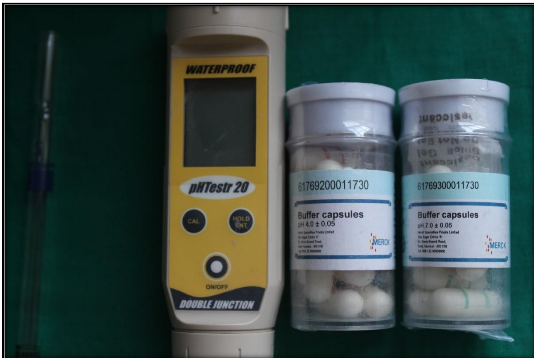
Figure 2: Hannah pH meter and buffer capsules (4 and 7)
