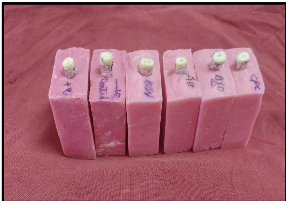
FIG: 10 TEETH MOUNTED IN ACRYLIC BLOCK FOR FRACTURE TESTING
