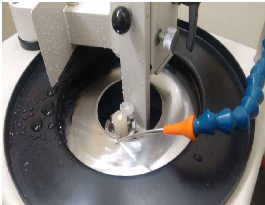
FIG 12: CROSS SECTION OF MIDDLE THIRD DONE WITH HARD TISSUE MICROTOME
