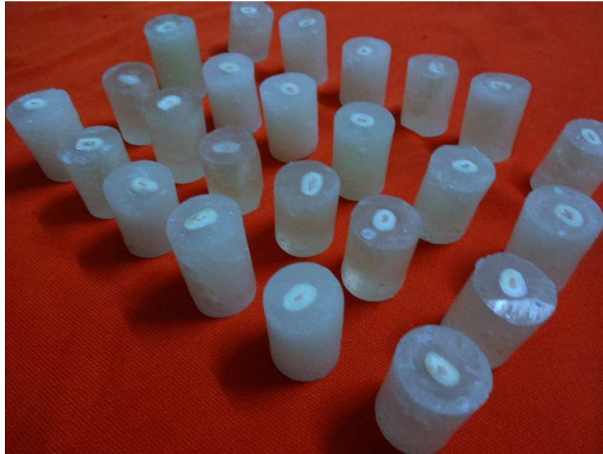
FIG 11: SAMPLES EMBEDDED IN SELF CURE ACRYLIC
