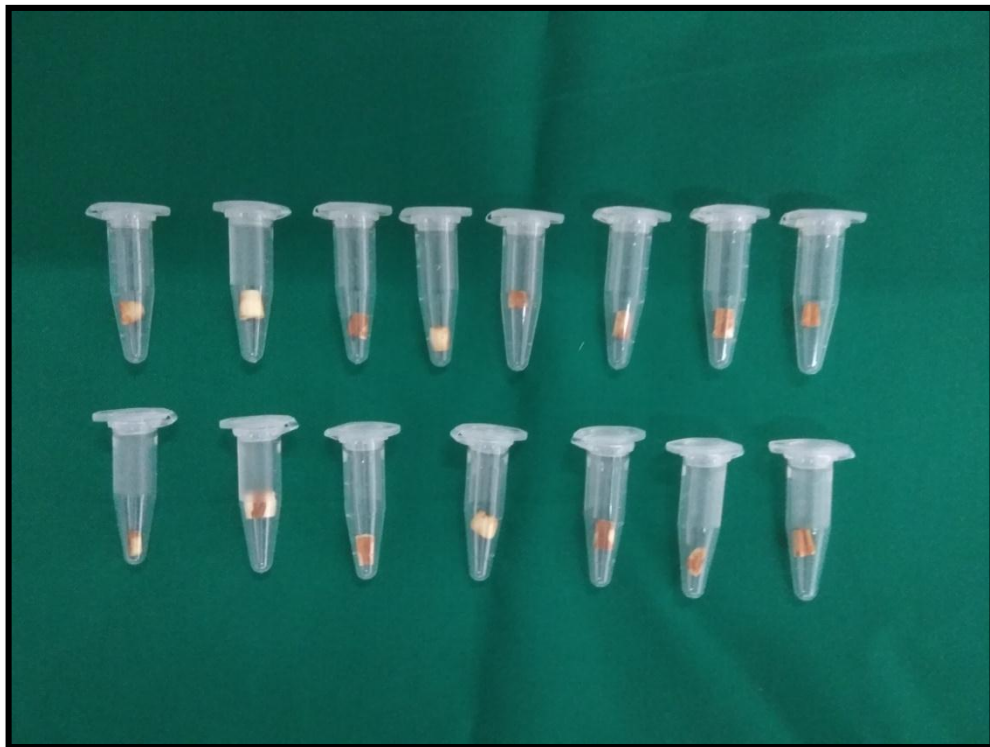
Figure 7: sample preparation after the placement of with curcumin modified MTA sealer for evaluating anti bacterial efficacy
