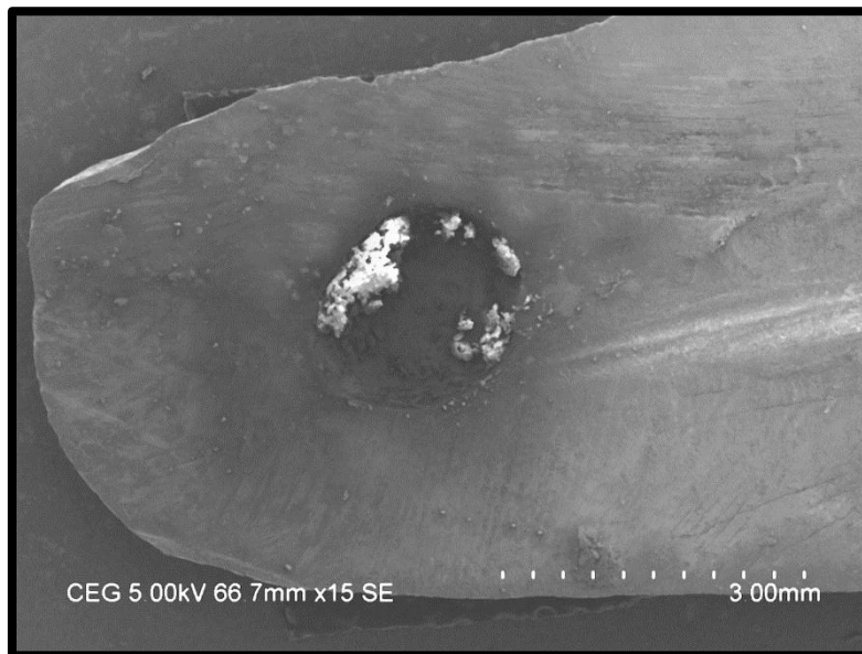
Fig 23: SEM image showing < 50% of depression filled with debris- score 2
