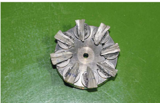
Fig 12 : Samples after sputter coating
