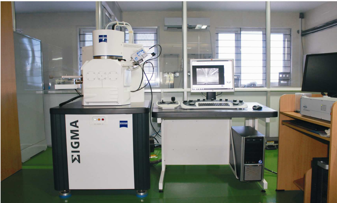
Fig 11 : Field Emission SEM Unit
