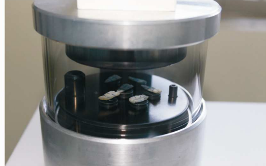
Fig 10 : Samples being sputter coated
