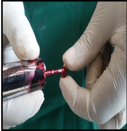
FIG 7 SPECIMEN COATED WITH NAIL VARNISH
