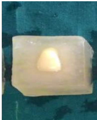
Figure : 4 Embedded crown in clear acrylic resin
