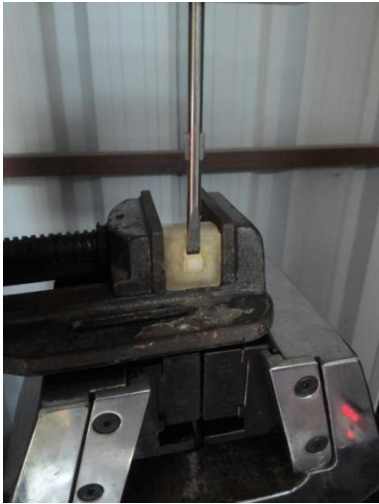
Figure : 12 Chisel placed at dentin – veneer interface
