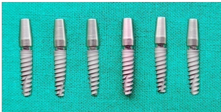
Fig.20: Group II test Samples( morse taper connection abutment)
