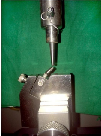
Fig16. After loading Adin internal hex implants in UTM 3345 with jig.
