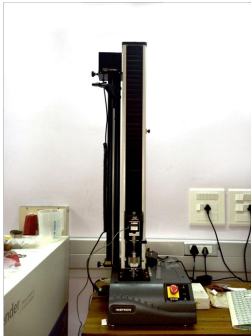
Fig.14: Custom made stainless jig positioning in static loading machine - instron 3345
