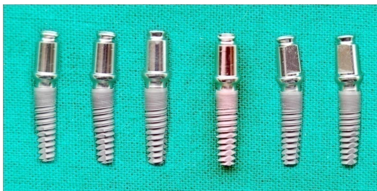
Fig.21: Group III test Samples(triconal connection abutment)
