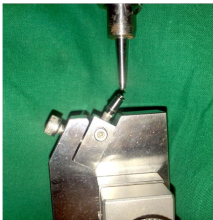
Fig18: After loading Equinox internal triconal implants in UTM 3345 with jig. .
