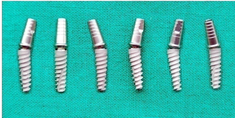
Fig.19: Group I test Samples ( internal hexagon connection abutment)
