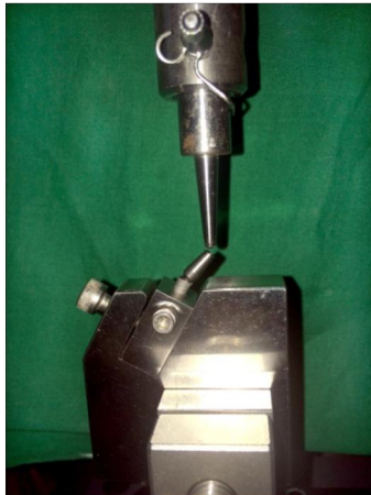
Fig17: After loading Adin Morse taper implants in UTM 3345 with jig.
