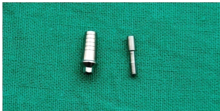
Fig.2: Prefabricated Titanium Dental Implant Abutment with internal Hexagon connection (Adin dental Implants ltd.Israel) .
