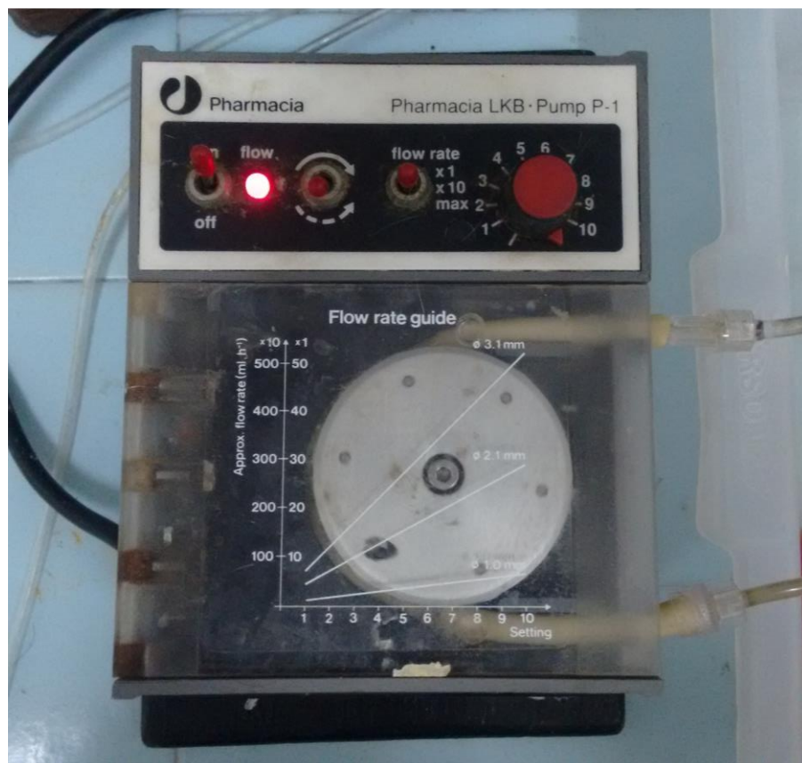
Figure 5: The peristaltic pump used for the experiments. It has a rotor with 6 rollers. The rollers compress the rubber tube and pump the fluid through the tube.
