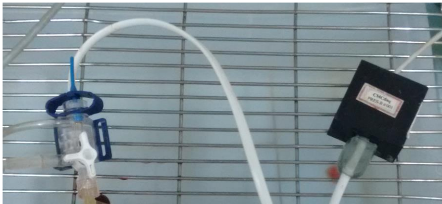
Figure 7: Pressure transducer and amplifier used for recording. Pressure transducer is the BP transducer used in ICU for intra-arterial BP monitoring. The amplifier and CMCdaq were developed by the Department of Bioengineering, Christian Medical College
