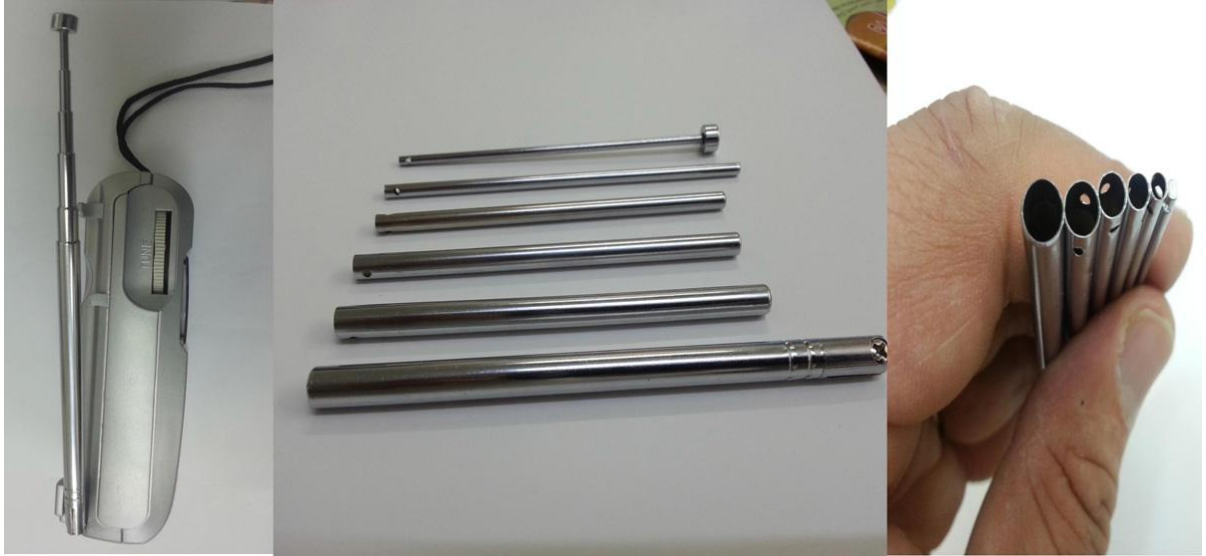
Fig 7 Usage of conventional TV Antenna in construction of TMA
