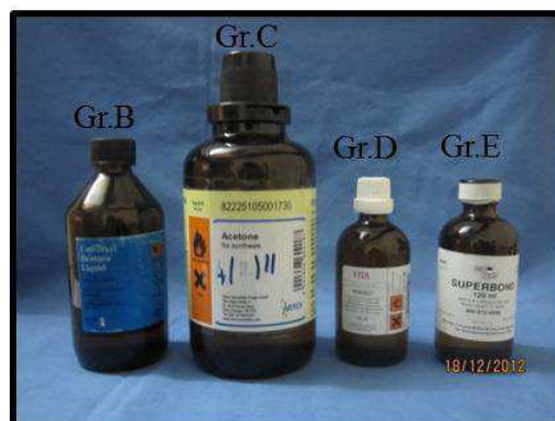
Fig-19 - Chemicals used for surface treatments.[from left to right] Group B- Heat polymerizing monomer; Group C - Acetone; Group D - Vitacoll bonding agent Group E – Super bond bonding agent
