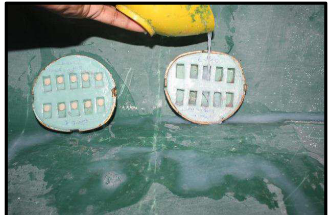
Fig-16 – Dewaxing with detergent boiling water
