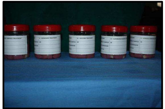
Fig-27 - Samples labelled and kept in water for aging (1 week)
