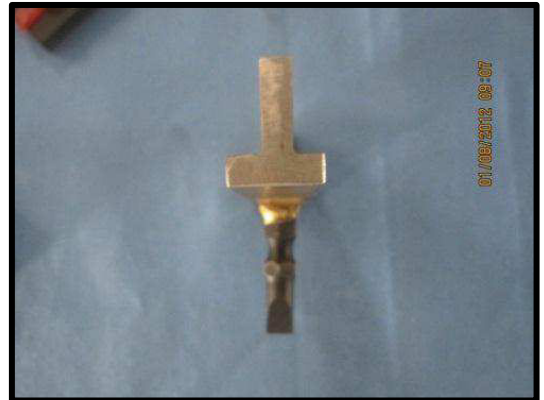
Fig-29 - Special chisel with 8mm diameter bevel
