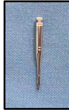
Fig-21 – Straight fissure tungsten carbide bur( RA 701L,SS White, Lakewood, NewJersy, U.S.A) For Group-D samples
