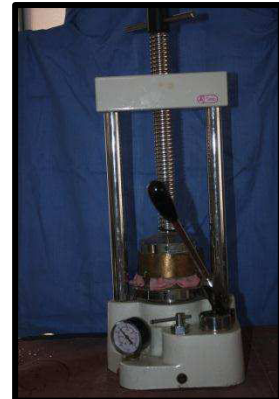
Fig-23 - Packing at 2000psi using pneumatic bench press
