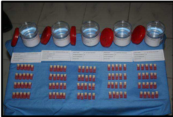
Fig-26 - Trimmed and polished test samples arranged in their respective 5 groups of 20 each
