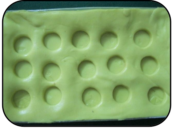
MOULD SPACE CREATED BY HEAT
