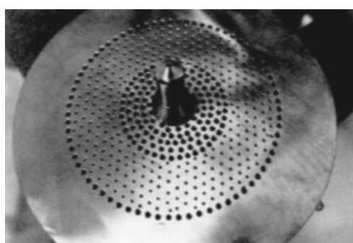
Air distributor or orifice plate of a Wurster coater.
