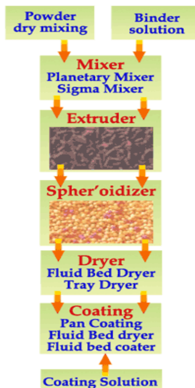
Fig:1.6 Scheme of pelletization stages in Extrusion and Spheronization.
