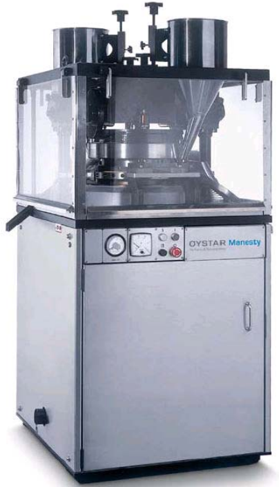
Figure 1: Double sided rotary press that can be tooled for Bi-layered compression of tablets; Oystar by Manesty.
