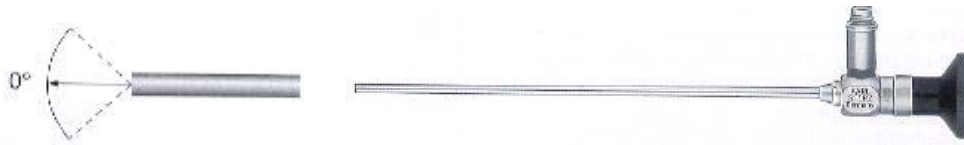
HOPKINS Straight Forward Telescope 0° , diameter 4mm, length 18cm, autoclavable , Fiberoptic light transmission incorporated
