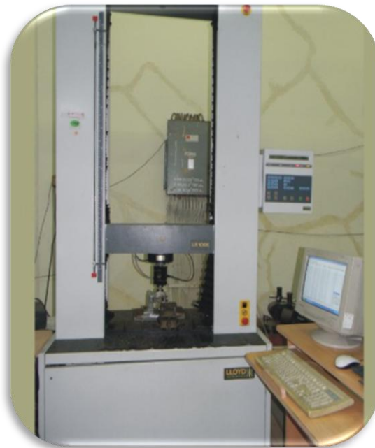
SHEAR BOND STRENGTH TESTING WAS DONE IN INSTRON UNIVERSAL TESTING MACHINE 1mm/ min (FIG.13)
