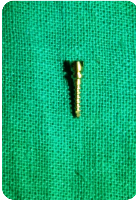
Fig 9- MSI's evaluated macroscopically for dimensional changes, distortion and fracture (control)
