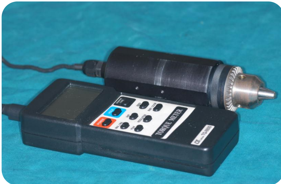
Fig 4- Digital torque driver with torque measuring meter. (Lutron TQ8800; Taiwan)
