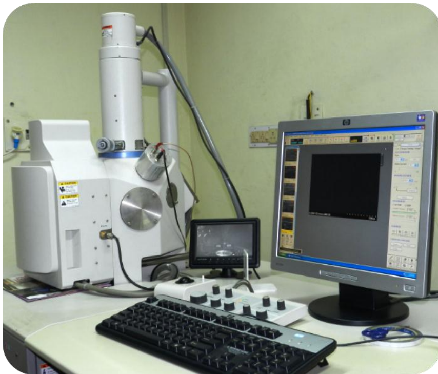
Figure 10: HITACHI, S3000N Scanning Electron Microscope (SEM) (Hitachi, Tokyo, Japan)
