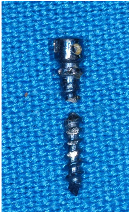
Fig 16- Macroscopic evaluation of a fractured MSI.
