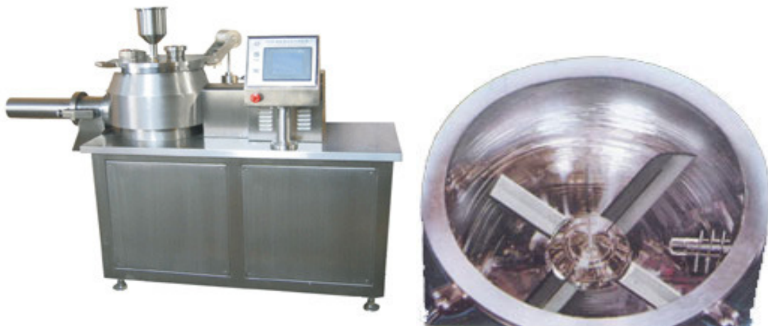
Rapid mixer granulator (RMG) with impeller and chopper
