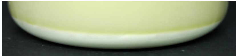
Figure 7.04: Separation of starch from Pisum sativum slurry
