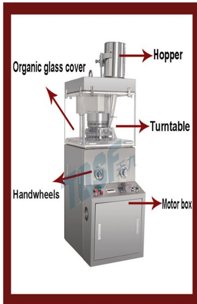
Figure 7: Direct compression technology – Tablet punching machine
