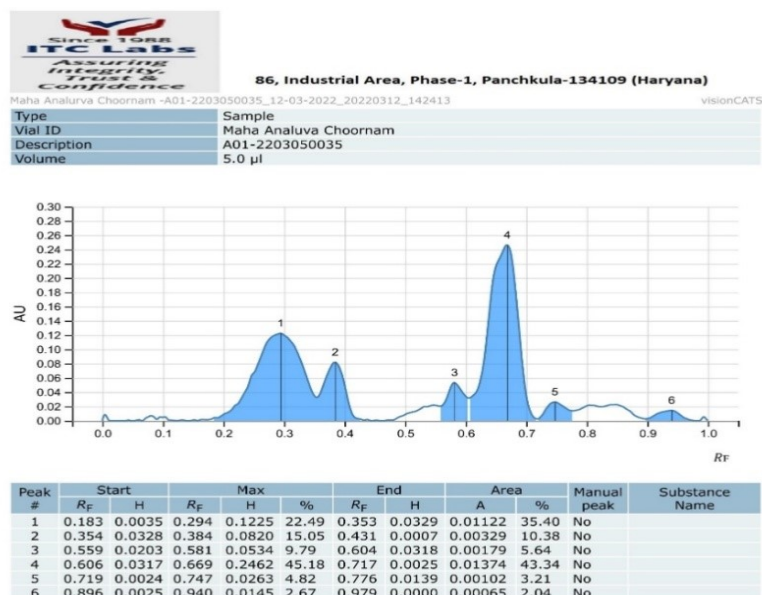
Figure: 4 Chromatographic identification & fingerprinting analysis of by HPTLC of Maha analuruva Chooranam
