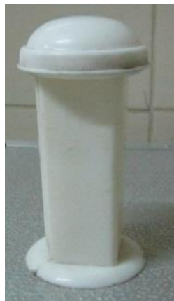
Fig showing the coupling jar which contains 10% isopropyl alcohol in which the slides are fixed
