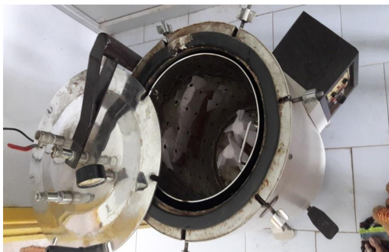
Fig No. 30 Sterilization of MGYP medium, Nutrient Agar medium, Potato Dextrose Agar medium by Autoclaving
