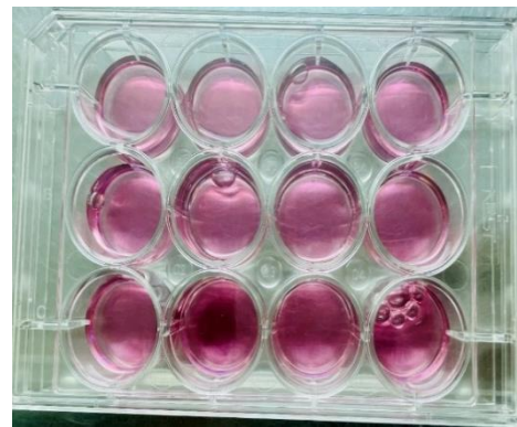
Figure23. Well plate that contain 2 ml of freshly prepared basal medium and 1 ml of hFOB cells
