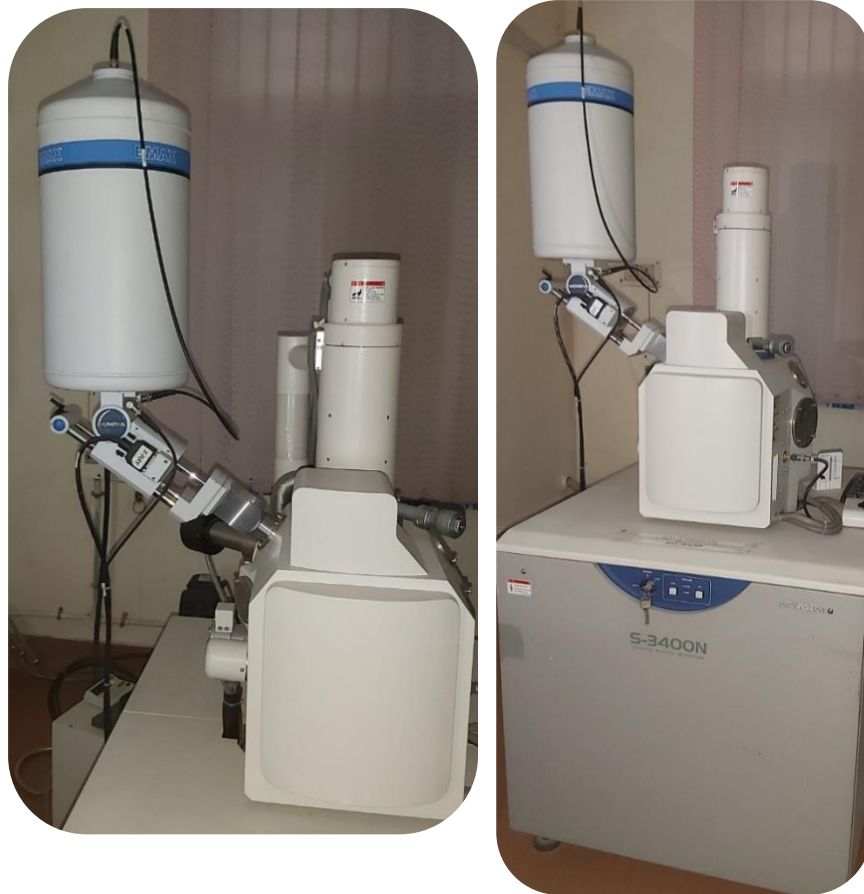
Figure 35. Scanning electron microscope to assess hFOB cells morphology.
