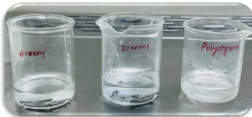
Figure 21. Titanium IZC mini-implants and polystyrene were immersed in 10 ml
