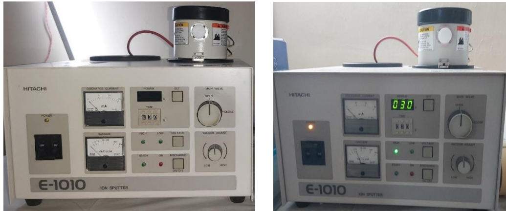
Figure 33. Samples were placed in a sputtering unit for 30 seconds for gold sputtering.
