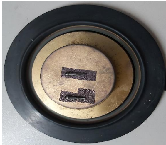
Figure 34. Gold sputter coated IZC titanium IZC mini-implants
