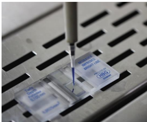
Figure 26. 10 \mu L of mixed suspension placed in hemocytometer using micropipette
