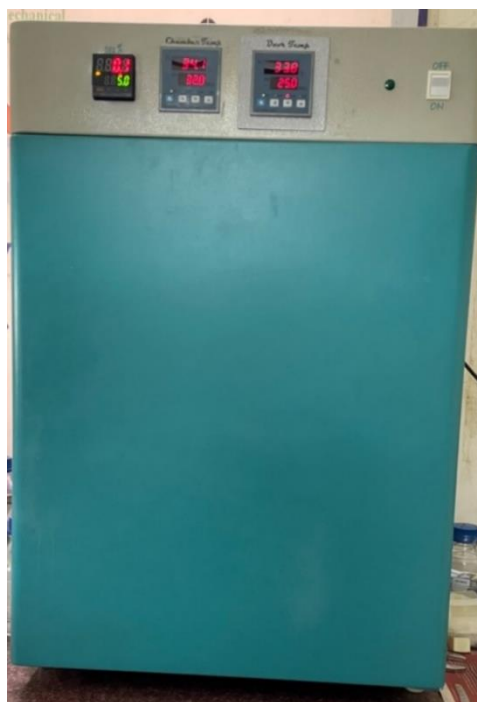
Figure 16. Incubator set with a temperature at 34°C
