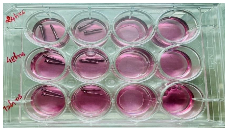
Figure 24. Titanium IZC mini-implants and polystyrene placed in well plate containing 2ml of basal medium and 1ml of cultured hFOB cells
