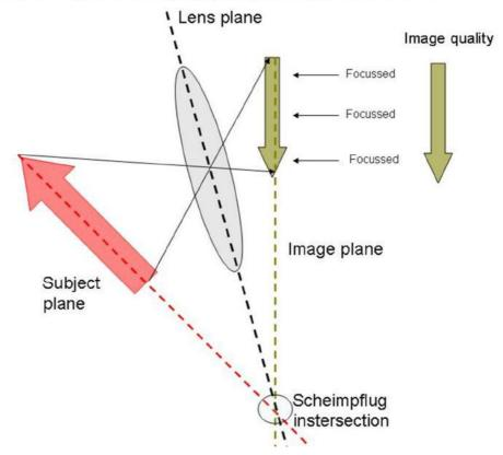
) Subject plane is still not parallel to image plane , however image plane is manipulated according to Scheimpflug principle : sharp focus overall
