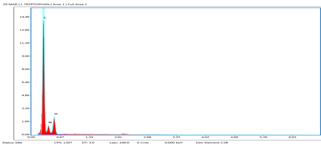
Figure No. 16: Energy Dispersive Spectroscopy graph of L Tryptophan
