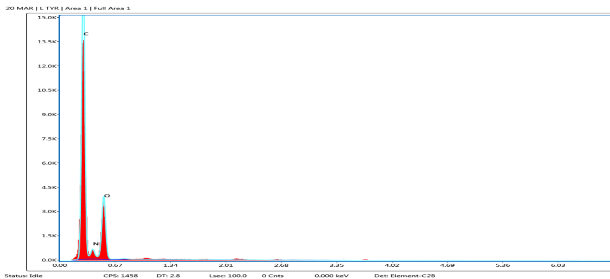
Figure No. 18: Energy Dispersive Spectroscopy graph of L Tyrosine
