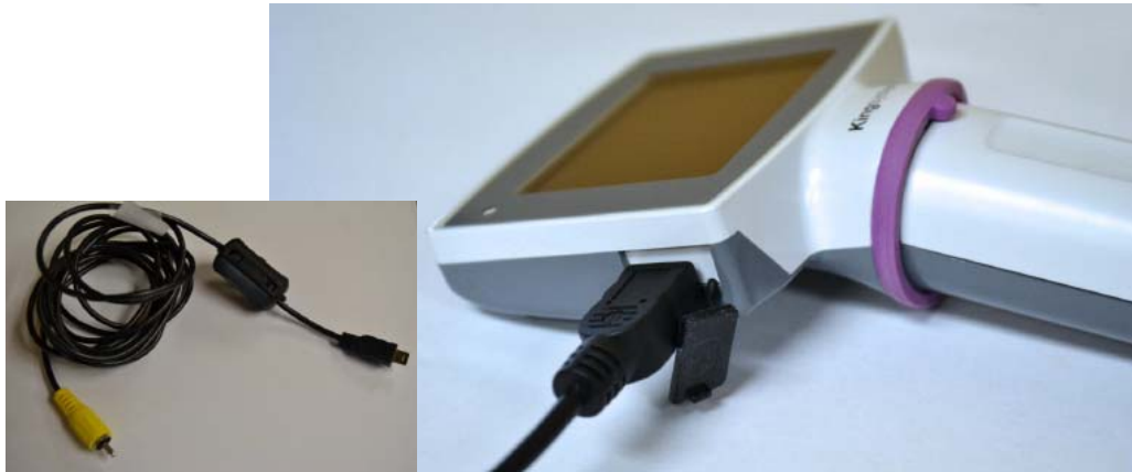
Fig 20: Video Output port and RCA Cable connector
