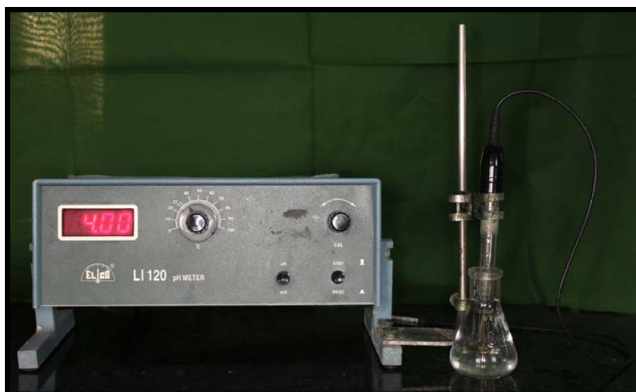
Figure 3: Prepared solution is checked for exact pH with pH meter
