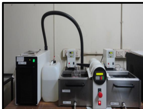
Fig.54: Thermocycling of test samples
