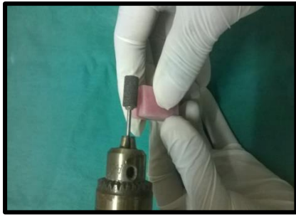
Fig.41: Finishing of the acrylic resin block
