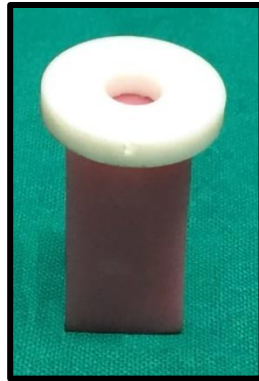
Fig.50: Assembly of Teflon jig- Acrylic resin block prior to adding silicone liner
