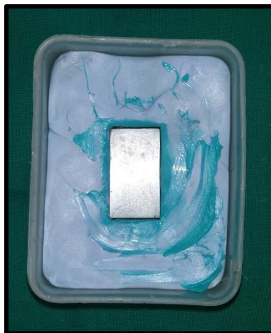
Fig.33: Seated stainless steel block into the mold space
