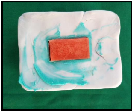
Fig.35: Modelling Wax poured into mold space
