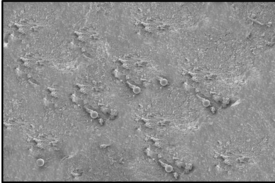
Fig.62 SEM photomicrograph of representative Group B (Sandblasted Group) debonded sample under 100x magnification
