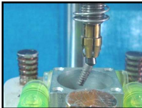
Fig.58: Positioning of implant-25 0 angled custom cast cobalt chromium abutment assembly in stainless steel block
