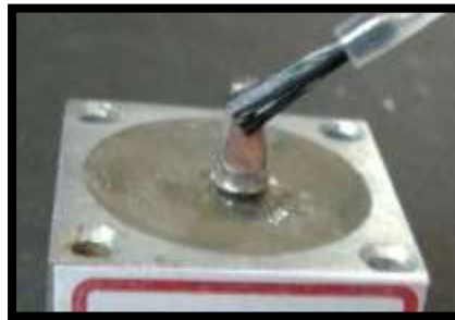
Fig.60: Application of die lubricant on the 25 0 angled milled premachined titanium abutment
