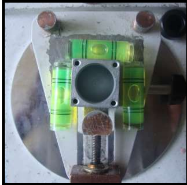
Fig.38: Surveying platform made parallel to floor using Spirit level indicators
