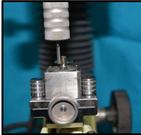
Fig.41: Milling of abutment
