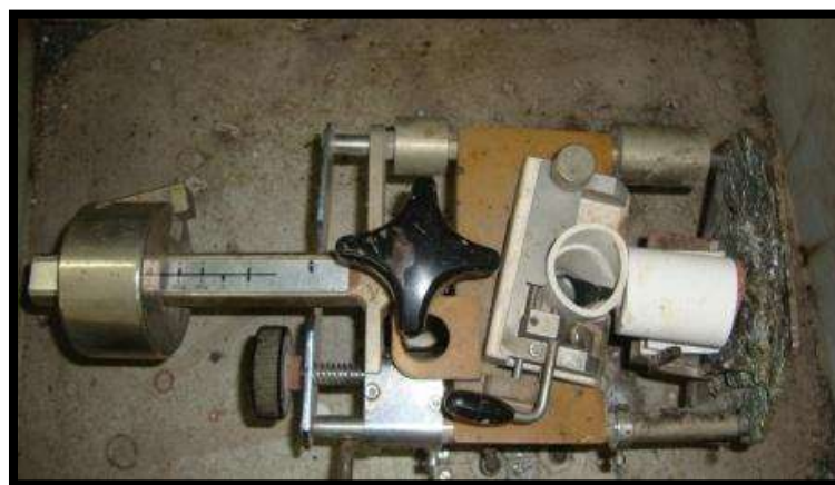
Fig.51: Casting done with Co-Cr alloy pellets using induction casting machine
