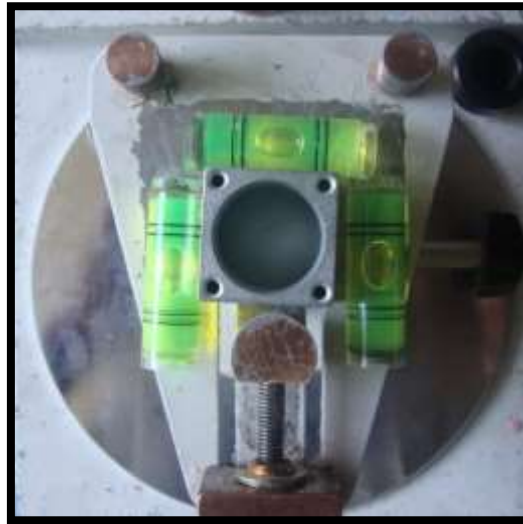
Fig.57: Surveying platform made parallel to floor using spirit level indicators
