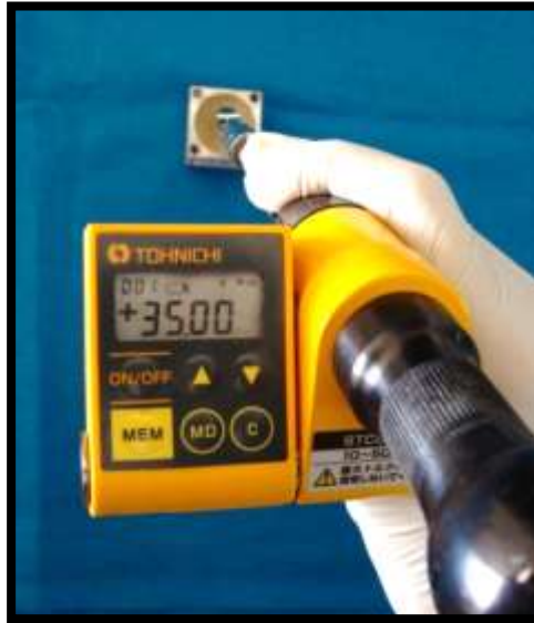
Fig.84: Retorquing of abutment screw to 35Ncm prior to cyclic loading
