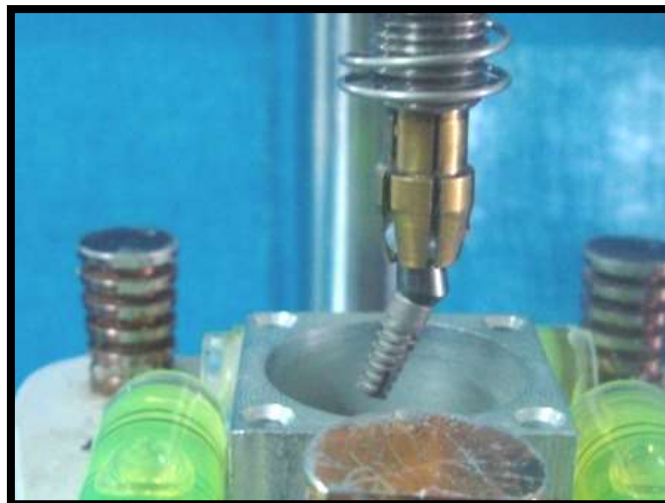
Fig.39: Positioning of implant-25° angled premachined titanium abutment assembly in stainless steel block
