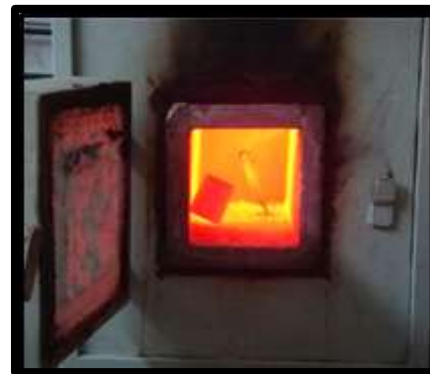
Fig.50: Burnout of pattern resin abutment
