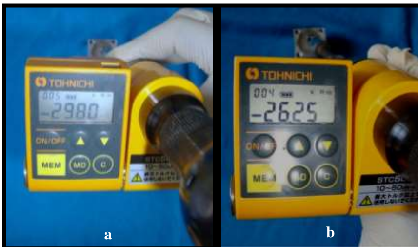
Fig.83 a: Measurement of reverse torque value before cyclic loading in Group I test sample
