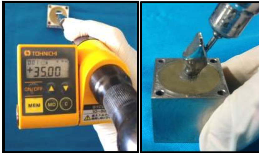
Fig.82: Torquing of abutment screws to 35Ncm
