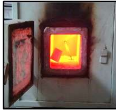
Fig.68: Burnout of wax pattern
