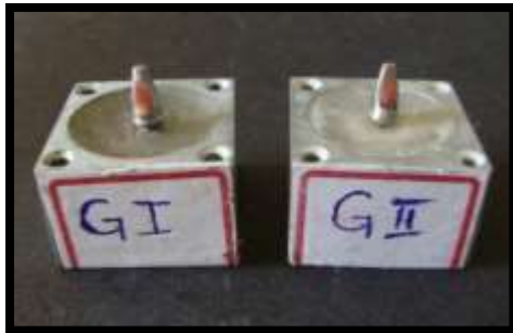
Fig.75: Sealing of abutment screw access with wax for Group I and Group II abutment
