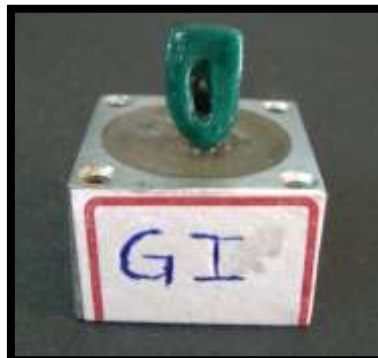
Fig.61: Wax pattern of central incisor with screw access hole on labial side for Group I test sample
