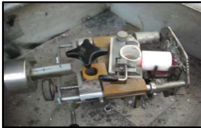
Fig.69: Casting of wax pattern with Ni-Cr alloy pellets using induction casting machine
