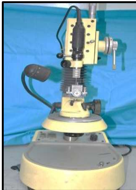
Fig.25: Milling unit with Surveyor
