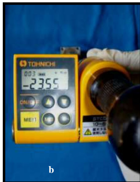
Fig.86a: Measurement of reverse torque value after cyclic loading in Group I test sample
