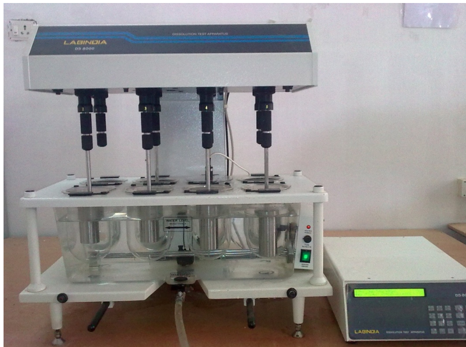
Figure no: 7 In vitro Drug release study using Dissolution apparatus USP VI
