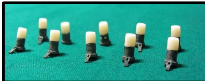
Fig.59: Porcelain veneered to DMLS Co-Cr alloy after laser etching (Group IV)
