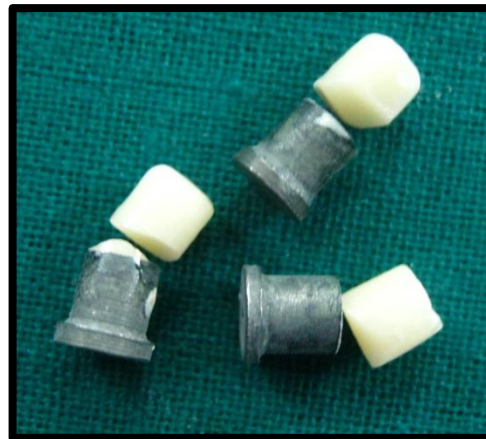
Fig.65: Debonded cast Co-Cr alloy-porcelain test samples after laser etching
