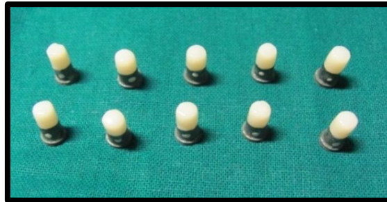
Fig.56: Porcelain veneered to cast Co-Cr alloy after sand blasting (Group I)
