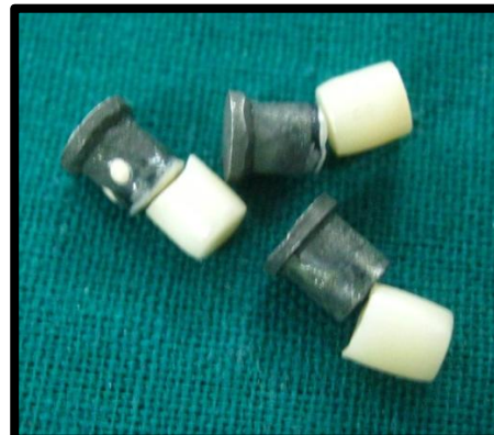
Fig.67: Debonded DMLS Co-Cr alloy-porcelain test samples after laser etching
