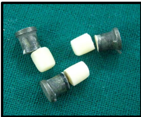
Fig.66: Debonded DMLS Co-Cr alloy-porcelain test samples after sandblasting
