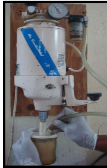
Fig.39: Vacuum mixing the investment
