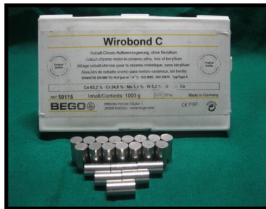
Fig.8: Co-Cr alloy pellets
