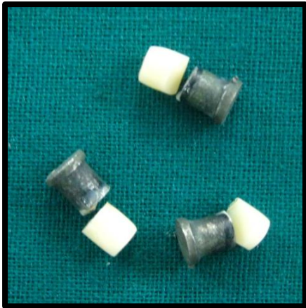
Fig.64 Debonded cast Co-Cr alloy-porcelain test samples after sandblasting
