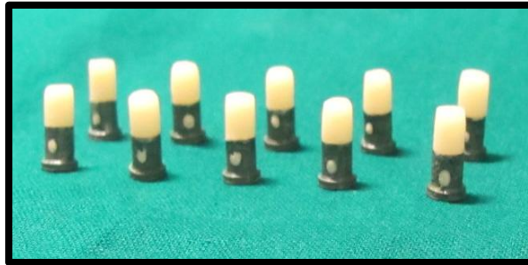
Fig.57: Porcelain veneered to cast Co-Cr alloy after laser etching (Group II)
