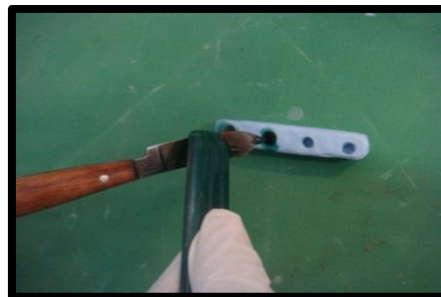
Fig.35: Preparation of wax pattern
