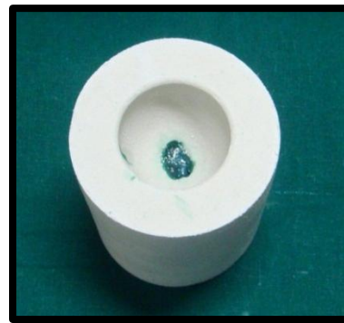
Fig.41: Wax pattern inside the set refractory mold
