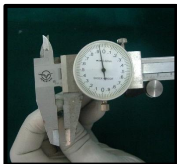
Fig.36: Checking dimensions of wax pattern
