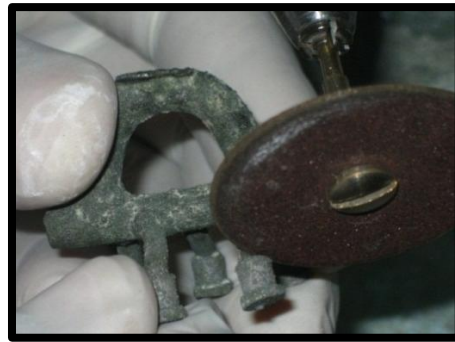
Fig.47: Cutting of the sprues
