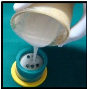
Fig.40: Investing the wax pattern
