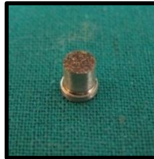
Fig.54: Nd:YAG laser etched sample
