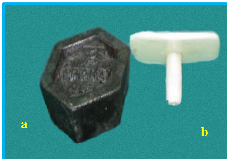
Fig. 14: Materials for load application to cemented cast copings
