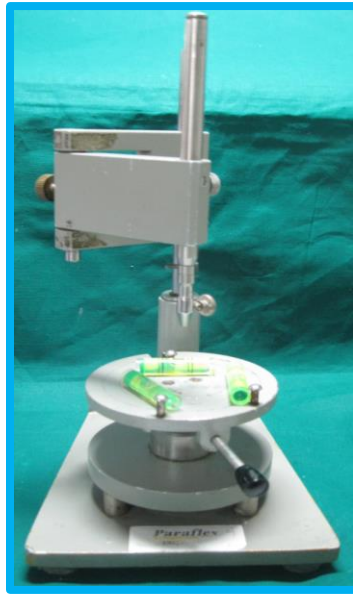
Fig.28: Making surveyor table parallel to floor with Spirit level indicators
