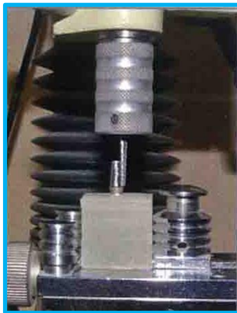
Fig.25: Milling of straight titanium implant abutment
