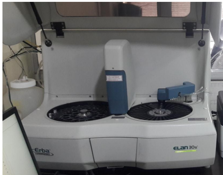
Fig 5-Fully automated equipment for Salivary estradiol analysis by ELISA method (Erba Mannheim,USA)
