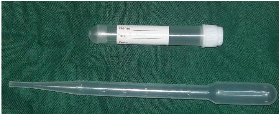
Fig 7-Disposable pipette (3ml) and storage vial (5 ml)
