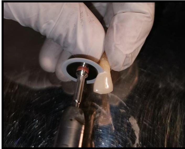
FIG:6 - DECORONATION OF SAMPLES WITH DIAMOND DISC
