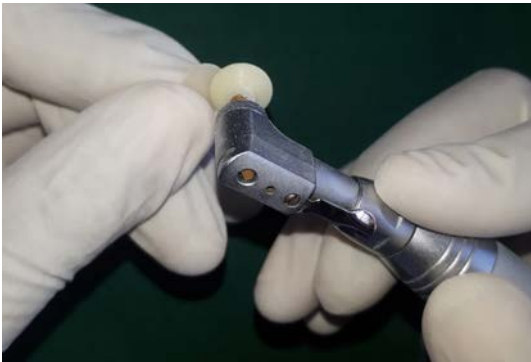
Fig-11: BOTH SURFACES OF COMPOSITE DISC ARE POLISHED WITH CAULK MICROPOLISHER IN G2,G3,G4&G5
