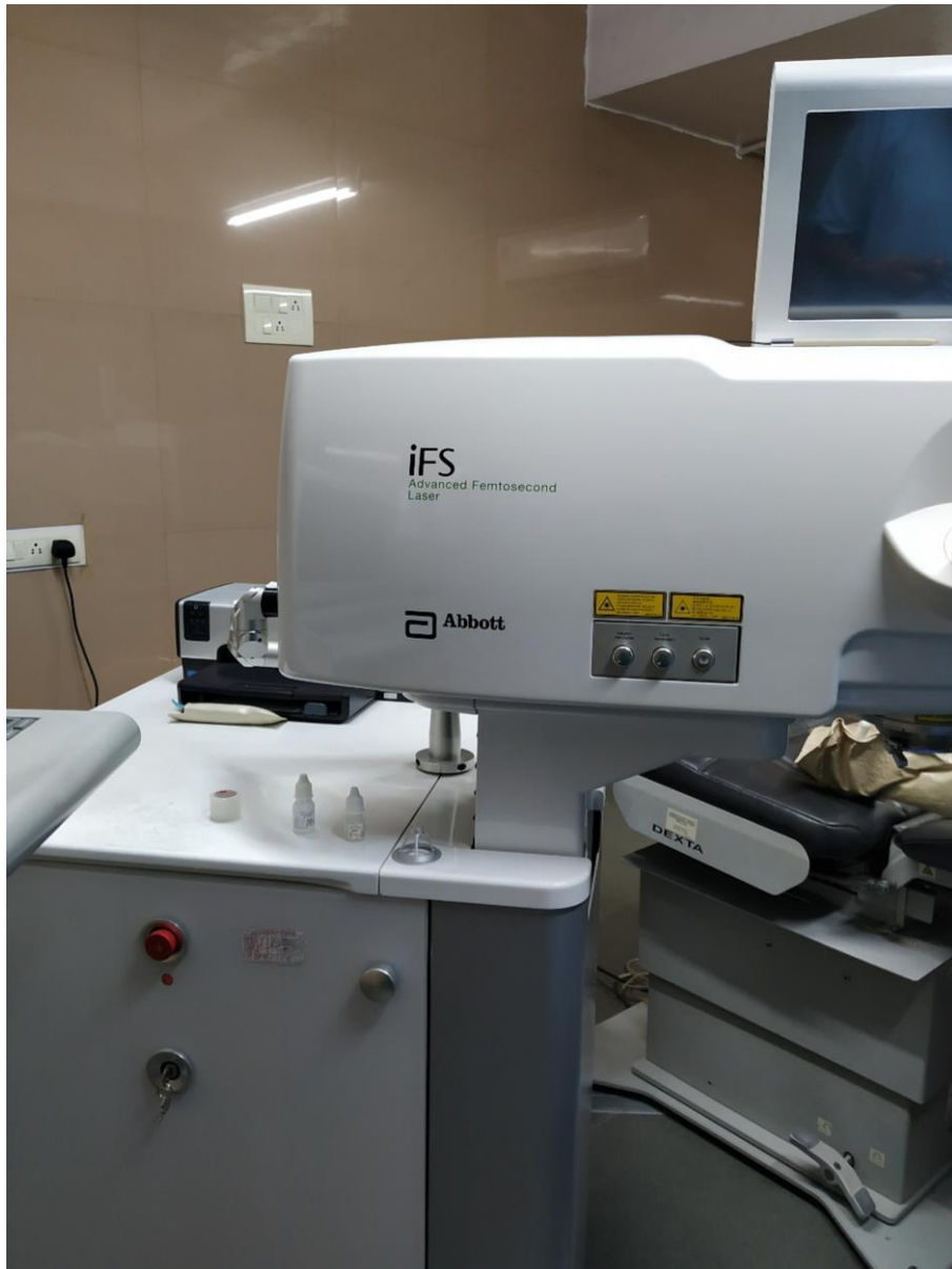
Figure 1.10: Intralase femtosecond laser for flap creation - iFS 150 kHz (Abbott Medical Optics Inc, Santa Ana, CA, USA)
